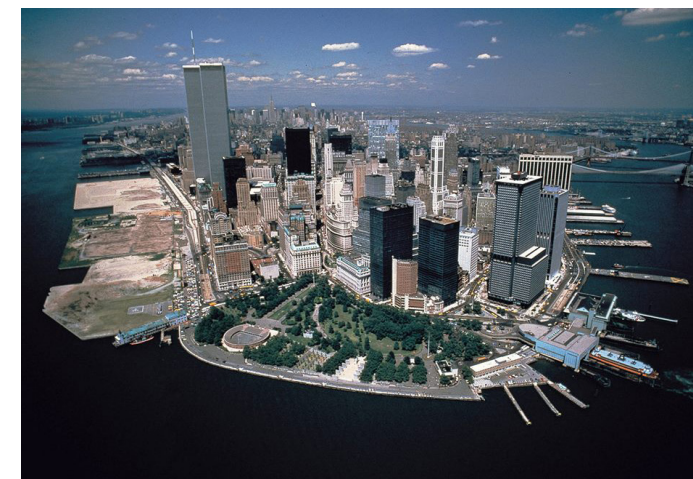
Precedent of land reclamation, or outboard, for Battery Park City (1973), not incorporated with resilient design at the time.
