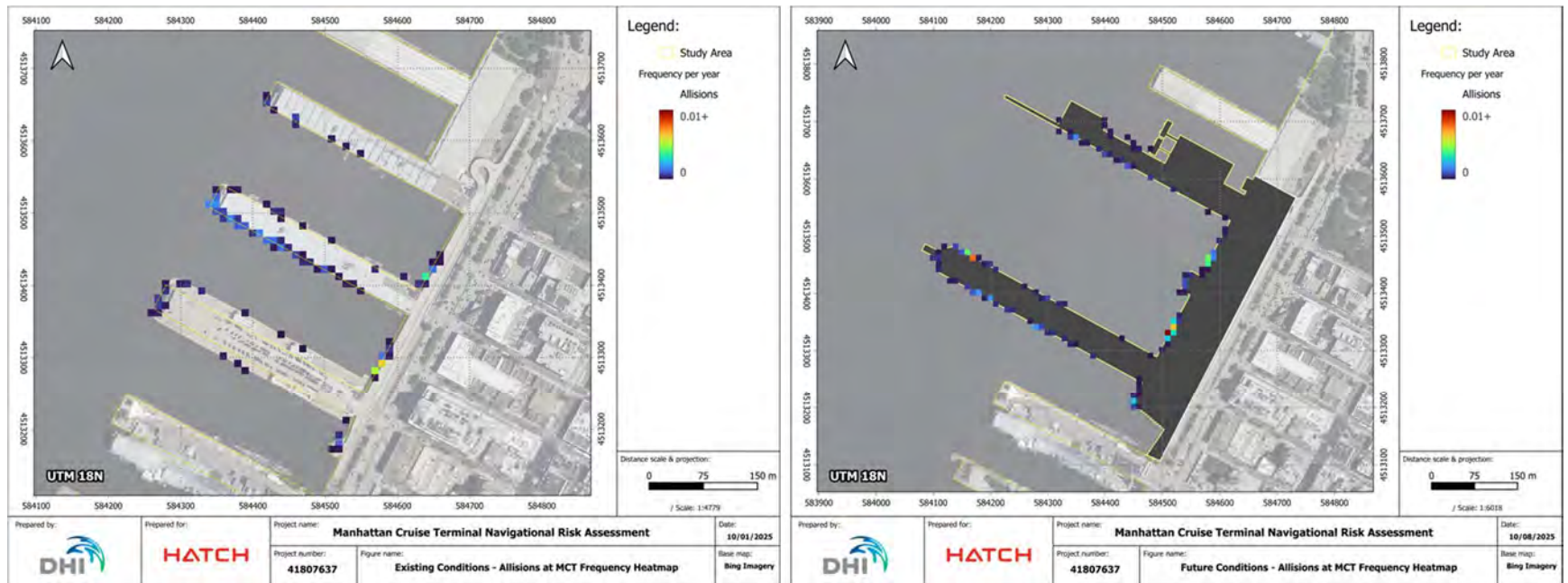
Figure 8-12: Existing (left) and Proposed Future (right) Allision Frequency Density Maps in at MCT
