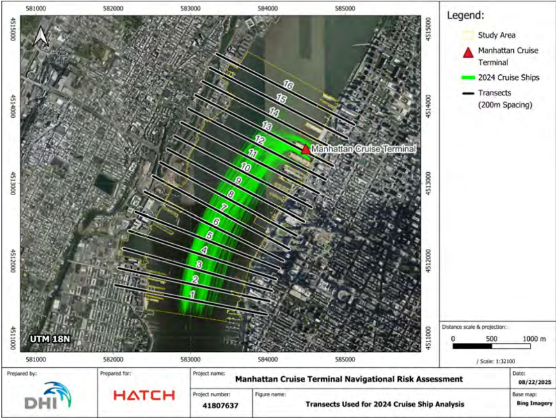
Figure H-1: 2024 Cruise Ship Call Tracks to and from MCT and Transects used for Speed Profile Analysis
