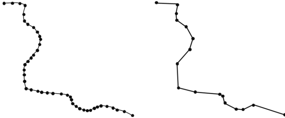
Figure K-1: Simplification of Raw AIS Tracks (left) to Characteristic Points (right)
