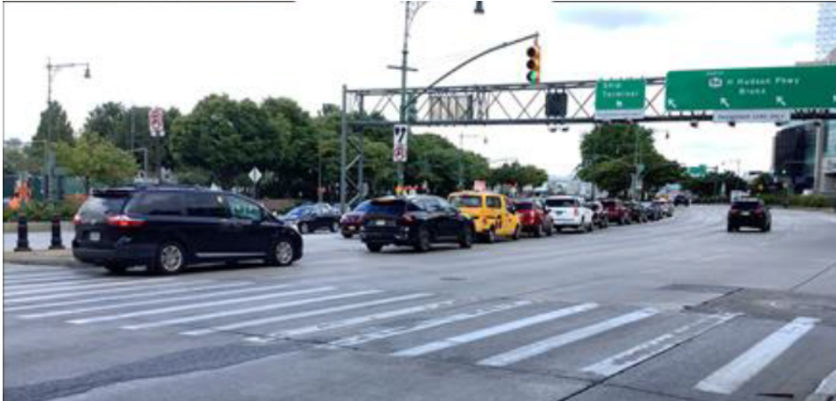
Figure 4: Spillback out of the left-turn bay into adjacent traffic on 12th Avenue
