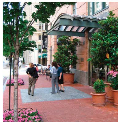
Lobbies should be emphasized with features such as special paving, a canopy, and planters
