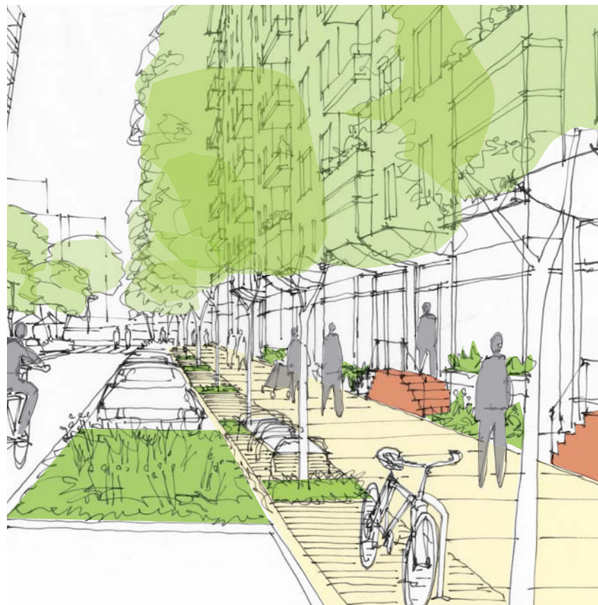
Figure 6. Rendering depicting LID systems that are incorporated into the parking lanes on the Residential Streets
