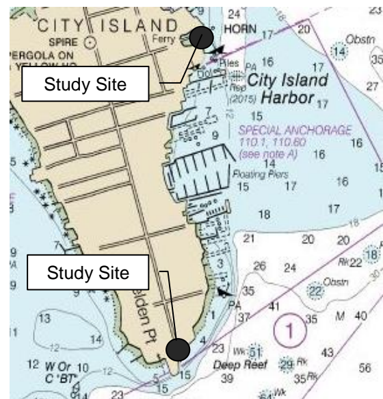
Figure shows water depth in feet at mean lower low water. NYC Ferry planning uses a minimum of 12 feet water depth when evaluating sites.
