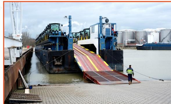
Roll-on/roll-off cargo ships that can be deployed for zero-emission freight transloading.
