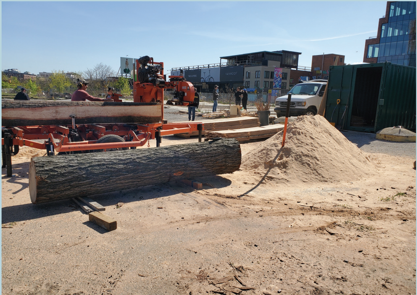
Brooklyn Woods trainees process milled lumber from salvaged logs in Greenpoint, Brooklyn. Source: NYC Parks
