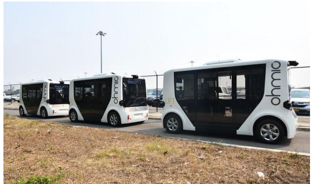
A pilot of an autonomous, all-electric passenger platoon made by Ohmio, a New Zealand-based startup. Photo: The Port Authority of New York and New Jersey
