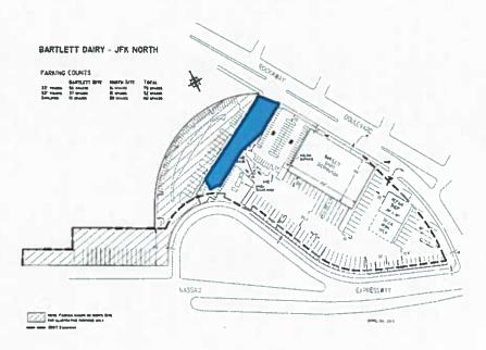
2) Con Edison Easement Area (shaded yellow) and Fenced in Area for Substation (shaded blue)
