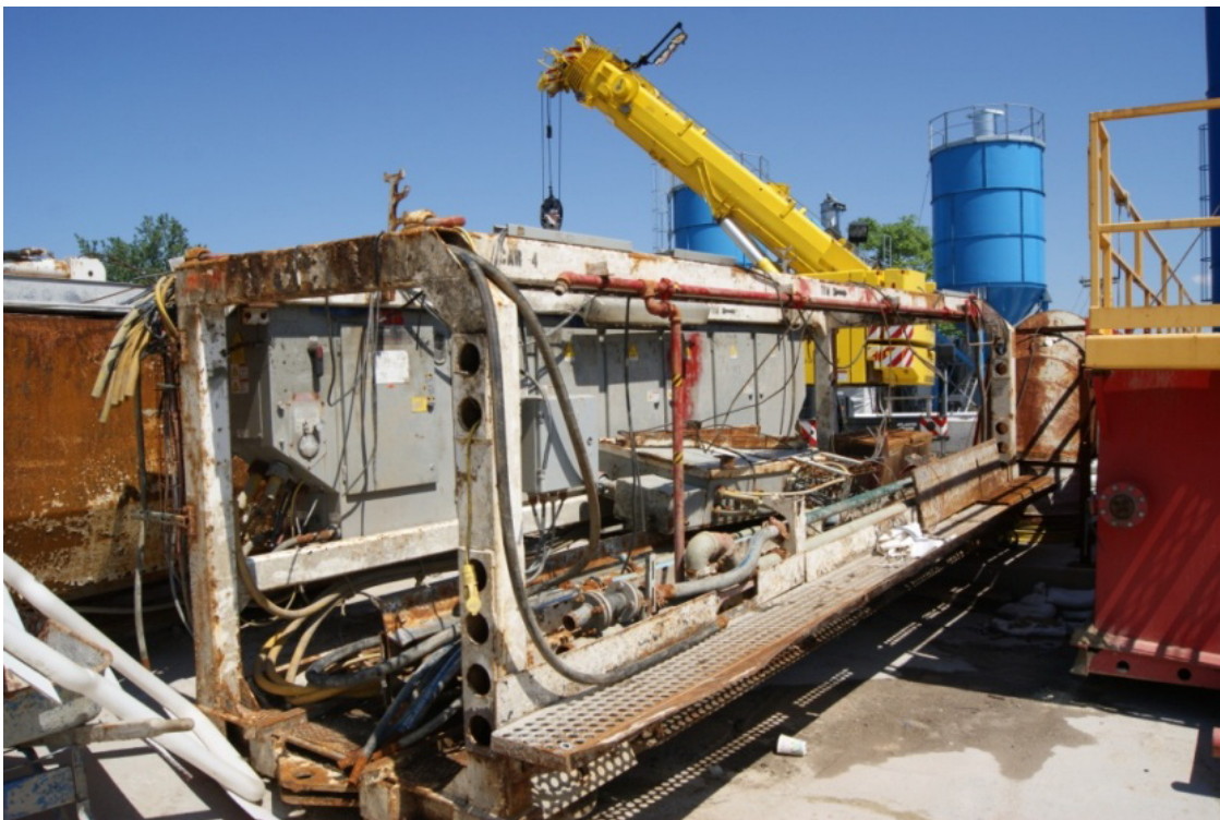
Sections of trailing gear removed from tunnel for repair (top and bottom photos)
